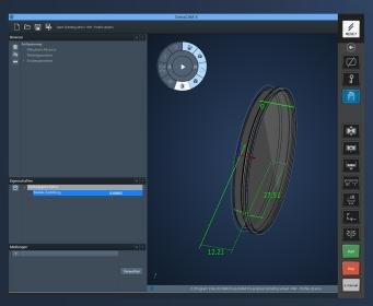
Using DressCAM X, dressing of profiled grindingwheels can be carried out easily and precisely directly on the machine control thanks to intuitive user guidance. The PROCESS-GENERATOR, the central control element in DressCAM X, guides the user automatically to the goal with just a few simple mouse clicks, even without a great deal of prior knowledge.
